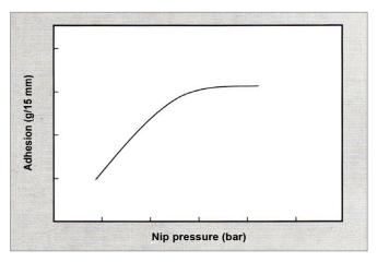
Figure 3: Effect of Nip Pressure on Adhesion of Extrusion-Coated LDPE to Porous and Non-Porous Substrates
