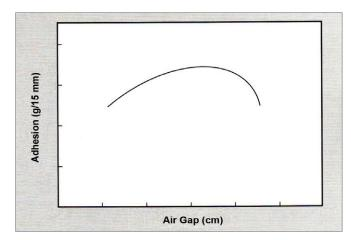
Figure 4: Effect of Air Gap on Adhesion of Extrusion-Coated LDPE to Non-Porous Substrates
