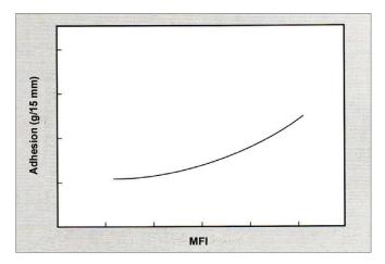
Figure 2: Effect of MFI on Adhesion of Extrusion-Coated LDPE to Porous Substrates
