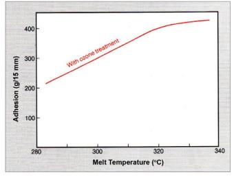
**Figure 1:** Effect of Melt Temperature and Ozone Treatment on Adhesion of Extrusion-Coated LDPE to Aluminium Foil
